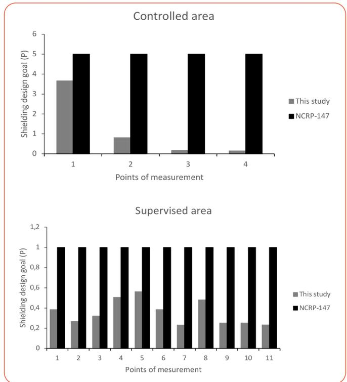
Figure 6. Comparison of this study shielding design goal with NCRP-147 limit for controlled and supervised area in centre B (The point 1-4 is A-D and 1-11 is E-O).
