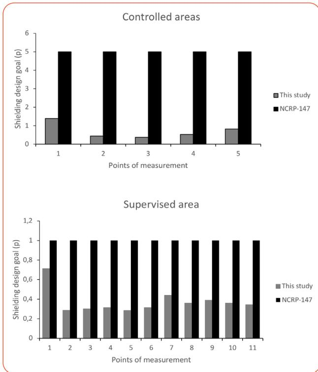
Figure 5. Comparison of this study shielding design goal with NCRP-147 limit for controlled and supervised area in centre A (The point 1-5 is A-E and 1-11 is F-P).
