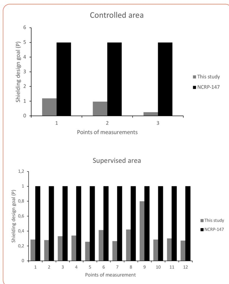
**Figure 7.** Comparison of this study shielding design goal with NCRP-147 limit for controlled and supervised area in centre B (The point 1-3 is A-C and 1-12 is D-O).
