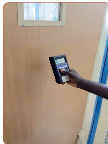
**Figure 4.** Shielded air kerma rate behind the lead screen.
