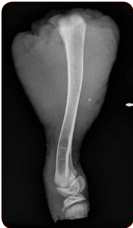
Figure 2c. CR lateral image of a chicken leg with a 3 mm sized glass piece inserted to the deep location and acquired using 50 kV and 3.2 milliampere seconds.
