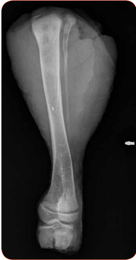
Figure 2a. Computed radiography (CR) anteroposterior (AP) image of a chicken leg with a 3 mm sized glass piece inserted to the deep location and acquired using 50 kV and 3.2 milliampere seconds.
