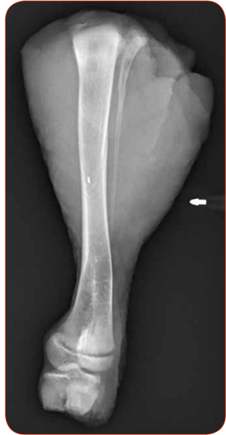
Figure 2b. Direct radiography (DR) AP image of a chicken leg with a 3 mm sized glass piece inserted to the deep location and acquired using 50 kV and 3.2 milliampere seconds.
