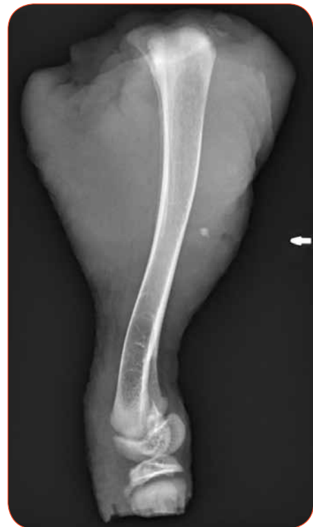
Figure 2d. DR lateral image of a chicken leg with a 3 mm sized glass piece inserted to the deep location and acquired using 50 kV and 3.2 milliampere seconds.
