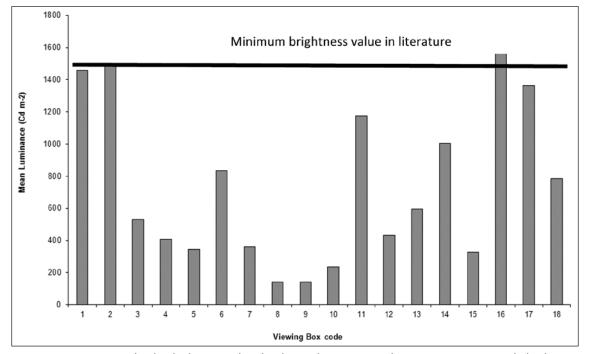
Figure 2: Comparison of individual viewing box brightness luminance with minimum recommended value in literature
