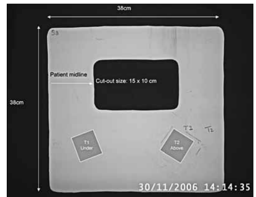
Figure 3: Shield S3 dimensions and dosimeter position.
