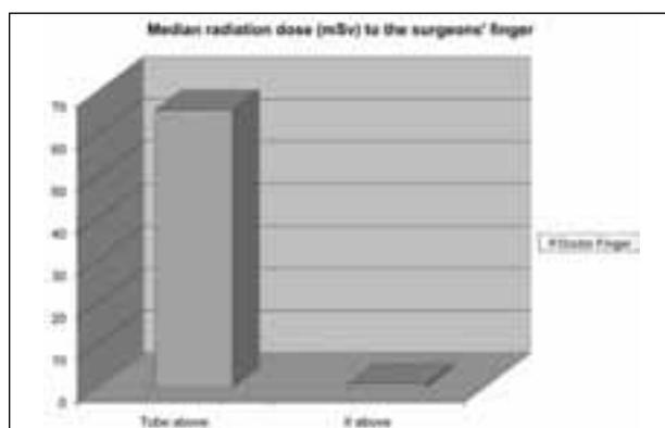
Figure 2: The finger dose values of the neurosurgeons with the x-ray tube and II respectively above the table
